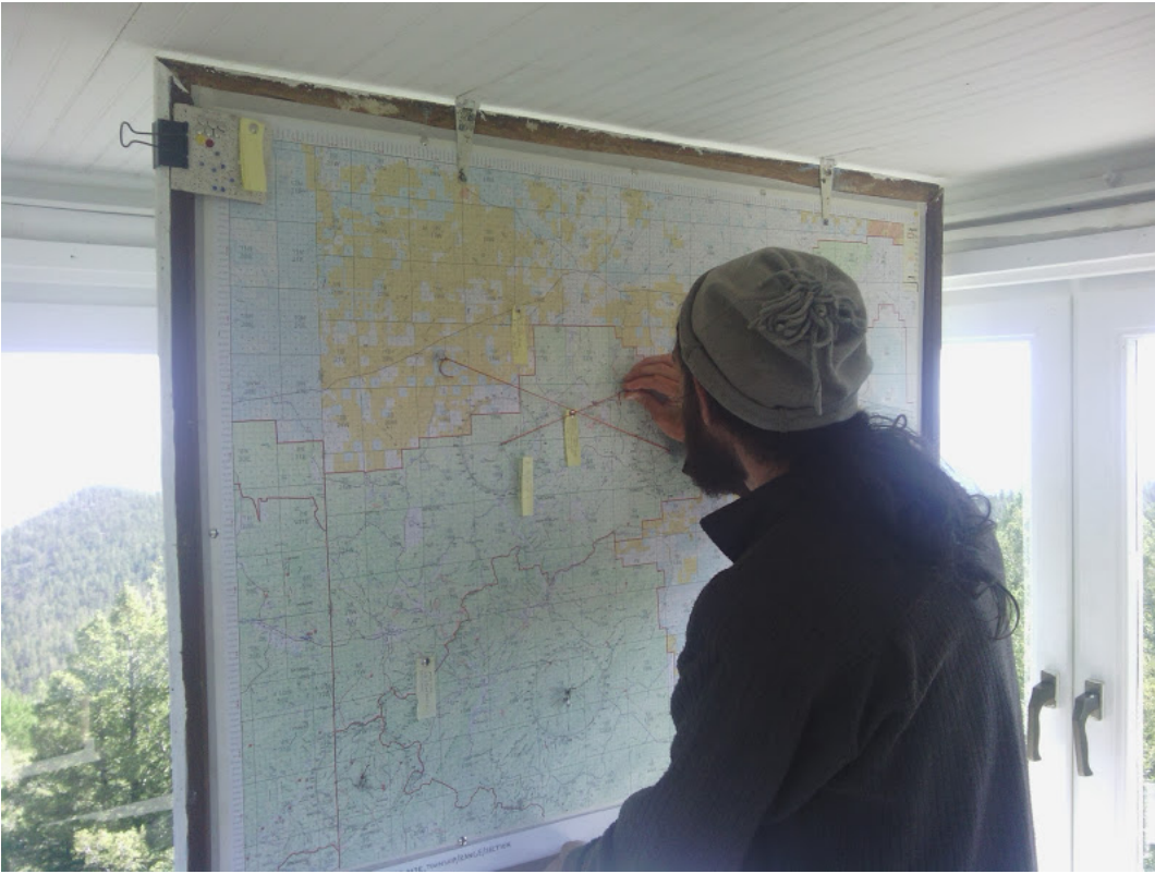
Triangulating fire location using bearings from two towers
